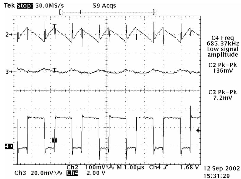
Figure 2-17 shows the output and input voltage ripple and main switching waveforms of the core regulator TPS54680/TPS54880 and I/O regulator TPS54610/TPS54810. The measurements are taken at  $V_I = 5\text{ V}$ ,  $V_O = 1.8\text{ V}$  (core),  $I_O = 6\text{ A}$  (core),  $V_O = 3.3\text{ V}$  (I/O),  $I_O = 0\text{ A}$  (I/O) and  $F_s = 700\text{ kHz}$  for both channels. For these waveforms:
