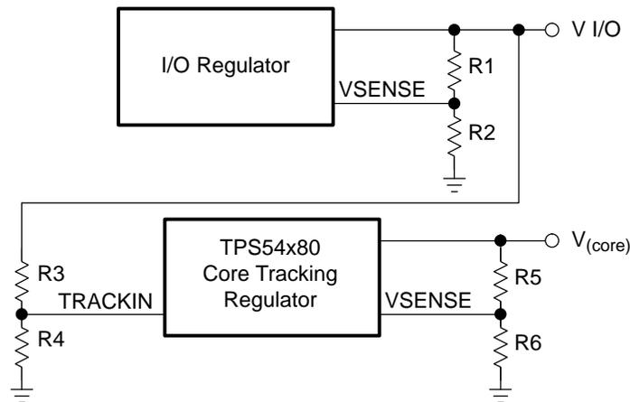
Implementation of different power sequencing techniques is based on proper resistor-divider ratio selection. The equations 1, 2, and 3 provide related ratios for different ways of power sequencing.
