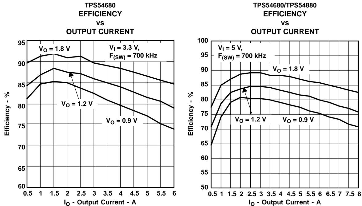
The input current, consumed by 3.3-V output regulator TPS54x10, is excluded from these data. The measurements relate only to the core voltage channel provided by tracking regulators TPS54680 and TPS54880. Efficiency is lower at higher ambient temperatures, due to temperature variation in the drain-to-source resistance of the MOSFETs. The efficiency is slightly lower at 700 kHz than at lower switching frequencies, due to the switching losses in the MOSFETs.
