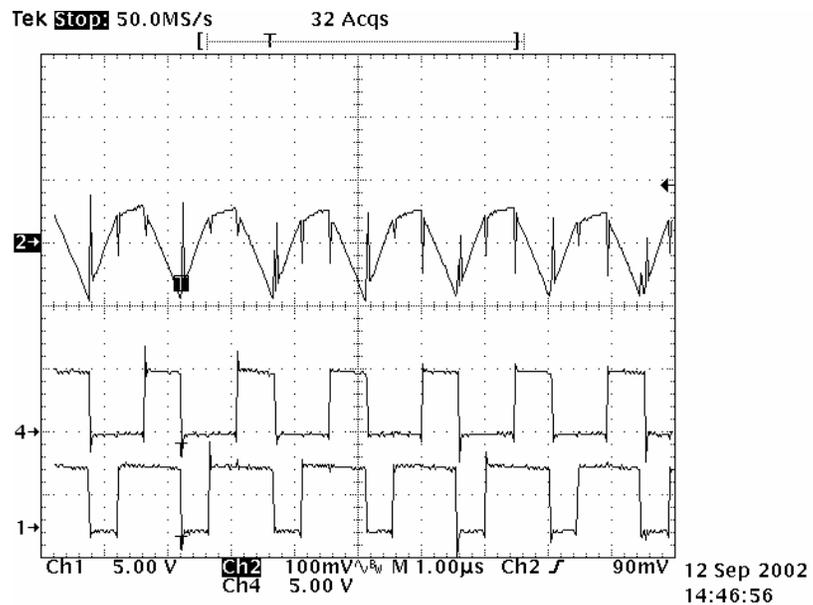
It can be seen that the input voltage ripple of synchronized regulators is 100 mV peak-to-peak, while the input voltage ripple of nonsynchronized regulators is 150 mV peak-to-peak. The ripple cancellation effect is the most significant when both regulators have roughly the same output current and the duty cycles complement each other.
