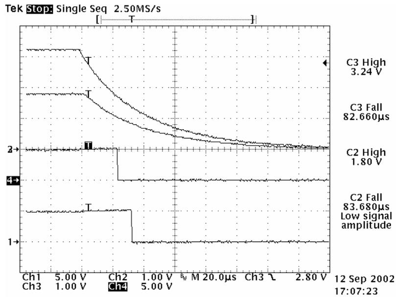
If jumper JP2 is set so that R2 is connected in parallel to R3, the core voltage rises first during power up, i.e. prior to the I/O voltage rise, and falls second during power down. The waveforms with this type of sequencing are shown in Figure 2-6 and Figure 2-7.
