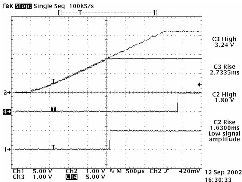
The powering down waveform, by using the ENABLE signal, is shown in Figure 2-3. During power down, the fall time of output voltage depends on the output capacitance and load resistance. In this case a very low resistance (0.5  $\Omega$ ) I/O output load has been selected to show the dynamic performance of the TPS54x80. It is seen that even if the I/O output voltage falls with the slew
