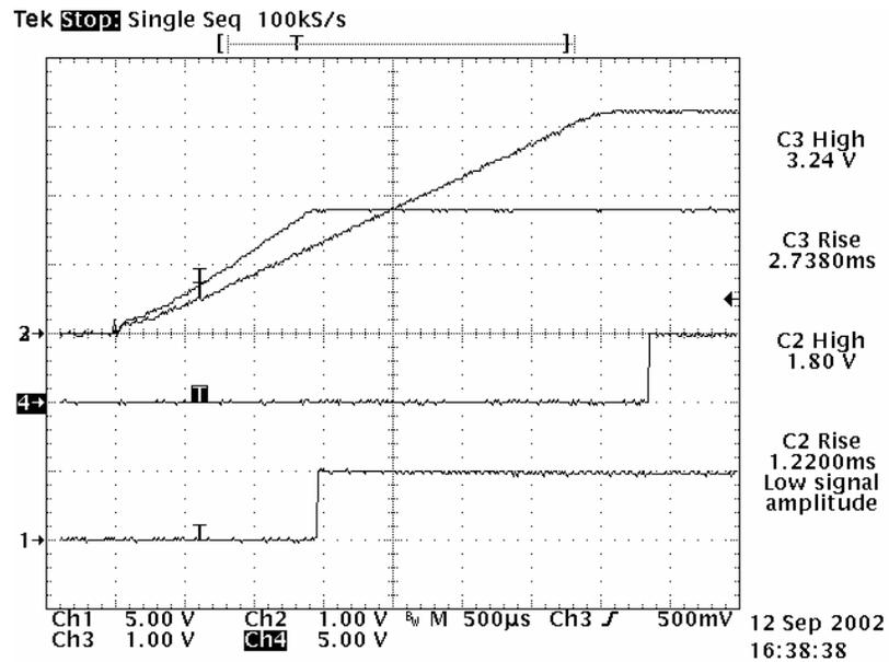
Figure 2-7. Powering Down With Core Voltage Falling Second
