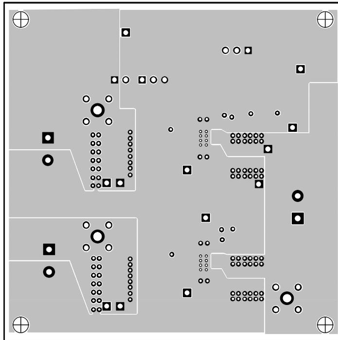
Figure 3-5. Bottom Side Layout (looking from top side)
