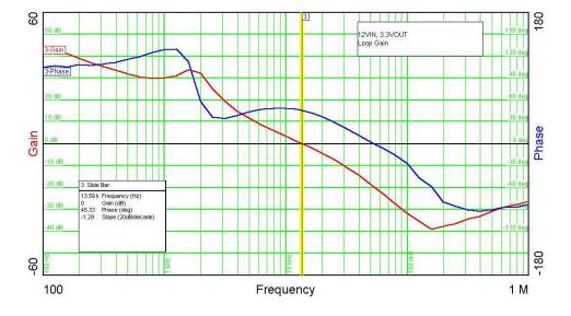
The figure below is the loop gain of the TPS54550 converter with max load. The bandwidth is 20 KHz, the phase margin is 82 degrees, and the gain margin is 28dB.
