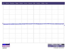
Output ripple/noise 1.5V output:
