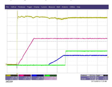
Output voltage turn-on response (traces, top to bottom, are: 1.8V, 1.5V, 1.25V, 1.2V):
