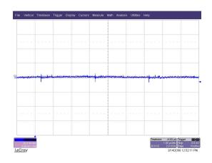
Output ripple/noise 1.2V output:
