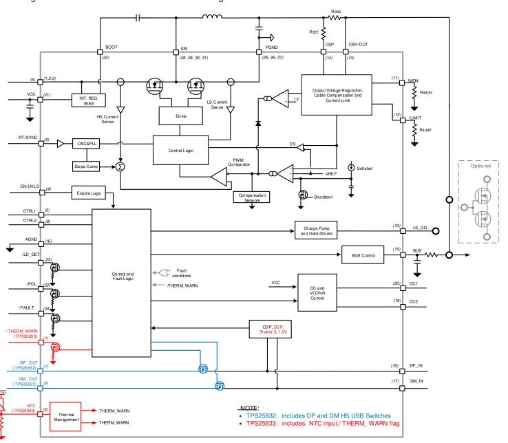
Figure 1-1. Functional Block Diagram
