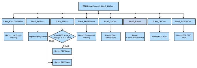
Figure 2. Fault Diagnostic Flow in Normal State
