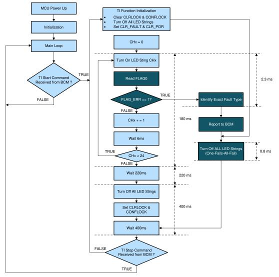
Figure 9. Implement One-Fails-All-Fail in Normal State
