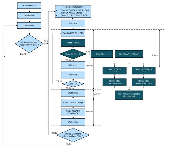
Figure 7. Identify Exact Fault Type in Normal State
