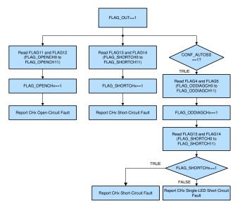
Figure 3. Output Fault Diagnostic Flow in Normal State
