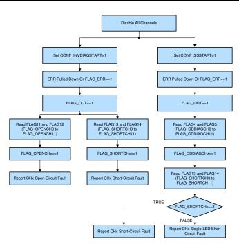
Figure 4. On-demand Diagnostic Flow in Normal State
