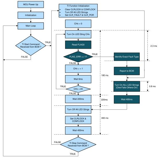
Figure 8. Implement One-Fails-Others-On in Normal State
