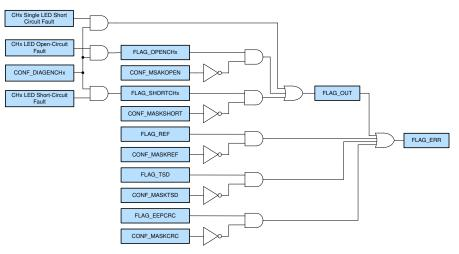
Figure 5. Diagnostic Enable and Fault Mask
