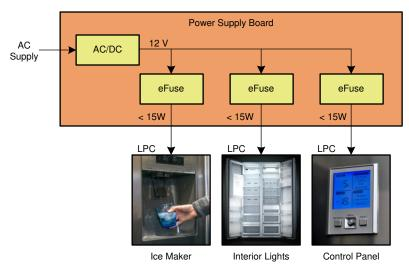
Figure 2. Example Block Diagram of Sub-circuits of a Refrigerator
