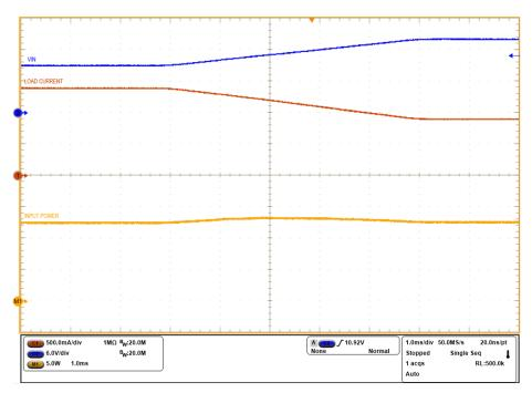
Figure 11. Test Result: Input Power Variation with Input Voltage with Current Injection Circuit
