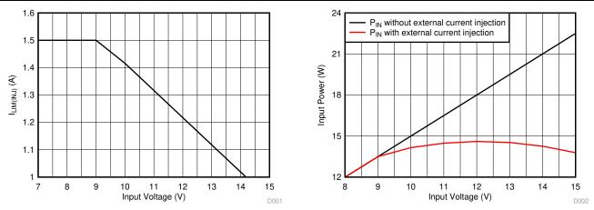
Figure 8. Current Limit with Current Injection Circuit vs Input Voltage
