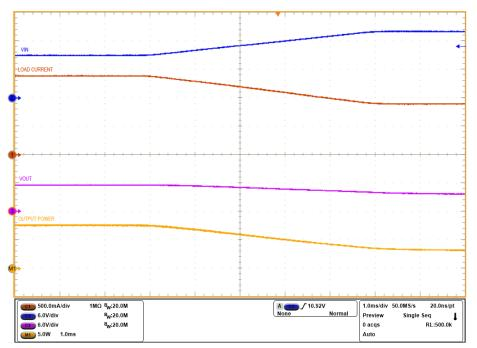
Figure 12. Test Result: Output Power Variation with Input Voltage with Current Injection Circuit
