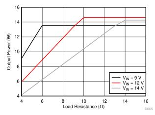
Figure 10. Output Power with Current Injection Circuit vs Load Resistance
