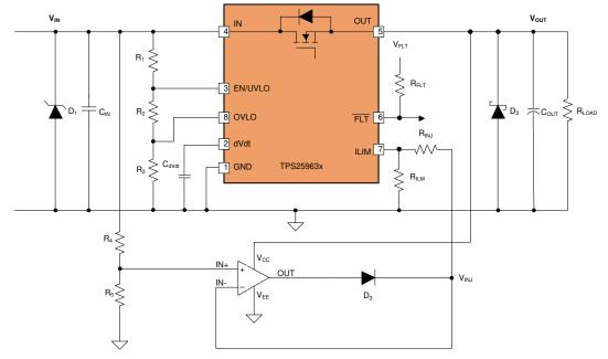
Figure 7. Application Schematic to Limit Power with Increase in Input Voltage
