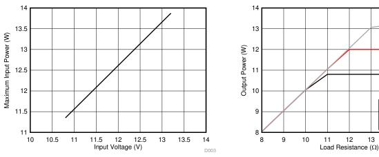
Figure 4. Maximum Input Power Limit vs Input Voltage
