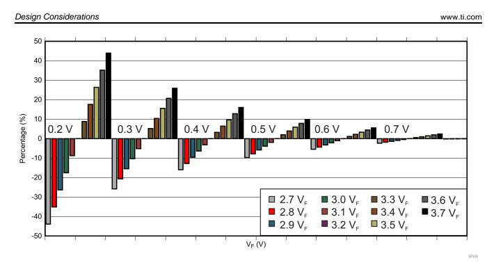
Figure 12. Error Trend With Lower V<sub>FB</sub>
