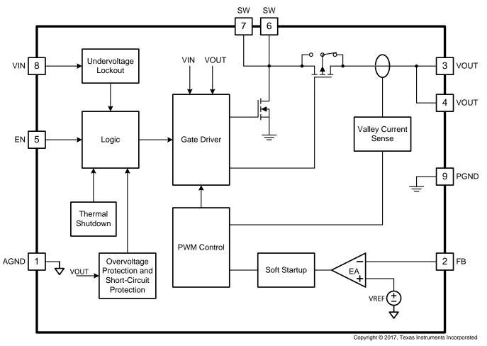
Figure 1. TPS61021A Internal Block Diagram
