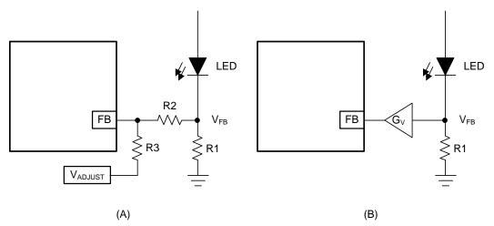
Figure 10. Using Voltage and Amplifier to Adjust V<sub>FB</sub>
