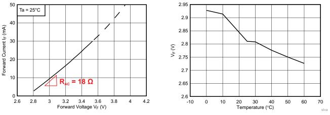
Figure 8. V<sub>F</sub> versus I<sub>F</sub>
