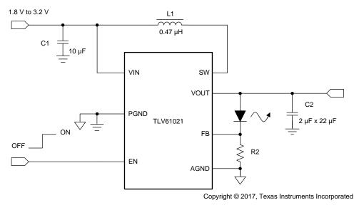
Figure 2. Direct Drive With FB Network
