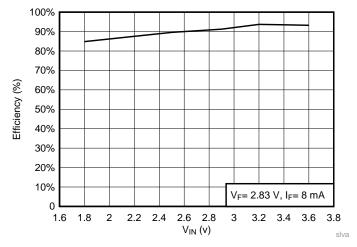
Figure 3. Load Efficiency With Different V<sub>IN</sub>
