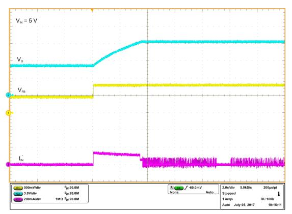
Figure 3. Start-Up Waveforms of VIN, IIN, VFB
