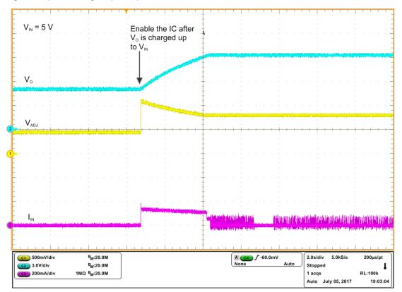
Figure 2. Start-Up Waveforms of V<sub>IN</sub>, I<sub>IN</sub>, V<sub>ADJ</sub>
