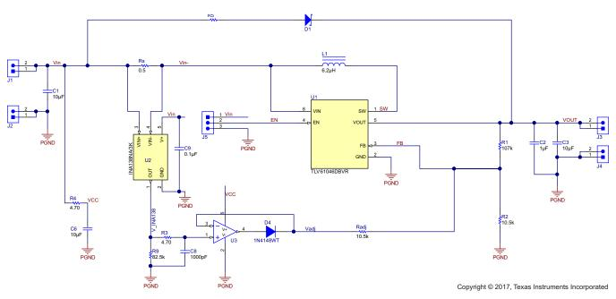
Figure 1. Schematic – Input Current Limit Solution
