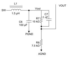
Figure 7. Feed Forward Capacitor for Higher Output Voltages
