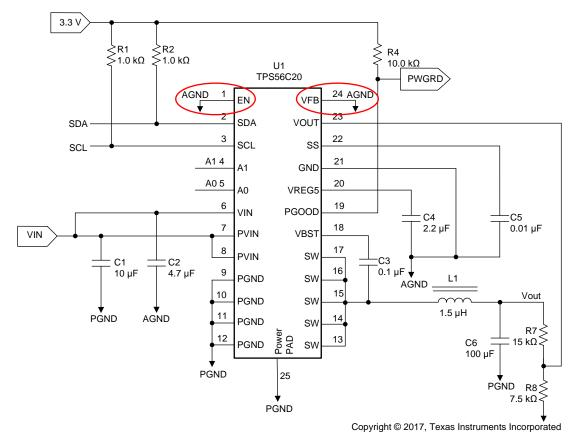
Figure 2. Proposed Circuit for Higher Output Voltage
