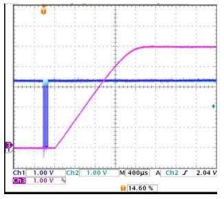
Figure 3. TPS56C20 Start Up (Vout = 5 V) With I<sup>2</sup>C
