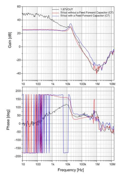
Figure 8. AC Sweep Results for Loop Gain and Phase Margin
