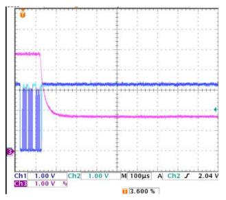
Figure 4. Output Voltage Change From 4.8 V to 1.8 V With I<sup>2</sup>C
