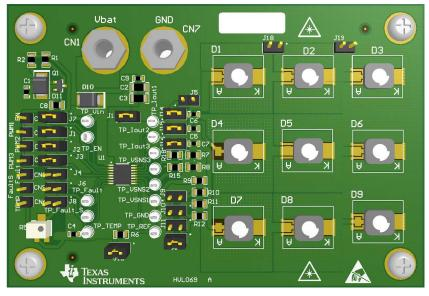
Figure 1. Top View of Test Board
