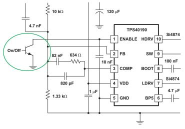
Figure 3. Discrete Transistor Buffer
