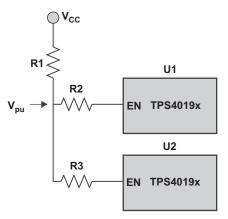
Figure 4. Block Diagram for Resistive Divider Method
