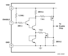
Figure 1. TPS4019x Enable Input Structure
