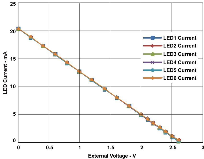
Figure 4. Actual LED Current vs External Voltage
