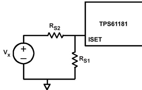
**Figure 1. TPS61181 Analog Dimming Configuration**
