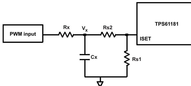
**Figure 2. RC Filter to get the Average Value of PWM Signal**
