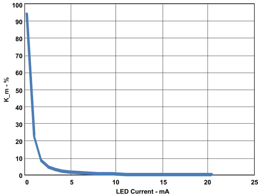
Figure 5. K<sub>m</sub> vs LED Current
