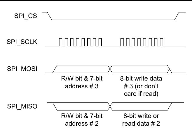
Figure 9-10. SPI Transaction #3 Without CRC
