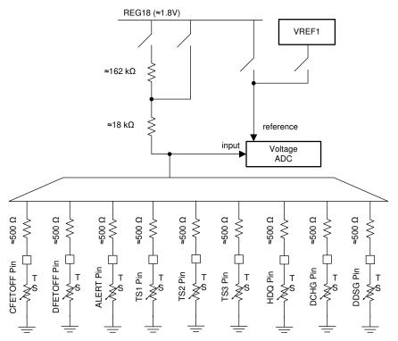
Figure 4-3. External Thermistor Biasing
