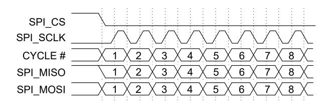
Figure 9-4. SPI with CPOL = 0 and CPHA = 0
