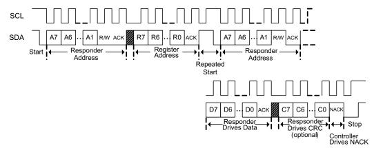
Figure 9-2. I<sup>2</sup>C Read with Repeated Start
