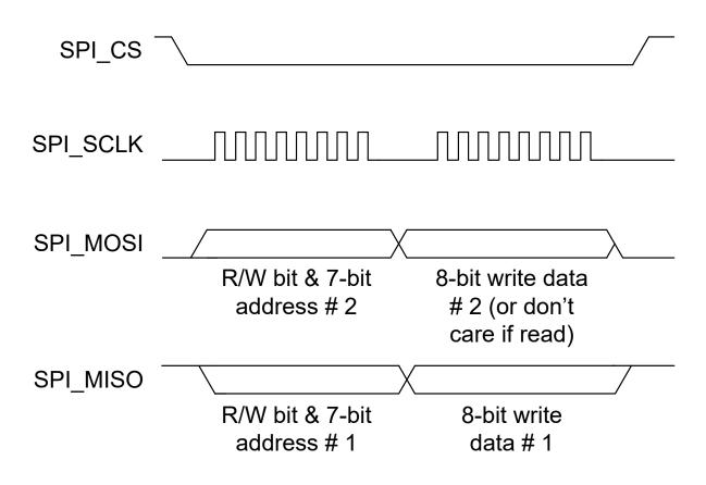
Figure 9-9. SPI Transaction #2 Without CRC
