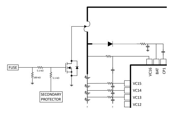
Figure 6-1. FUSE Pin Operation
