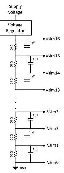
Figure 4-4. Example Fixture for Cell Offset Calibration
