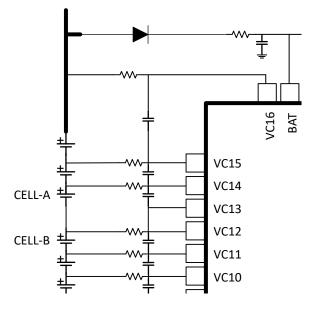
Figure 4-2. Terminating an Unused Cell Input Pin
