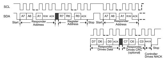
Figure 9-3. I<sup>2</sup>C Read Without Repeated Start
