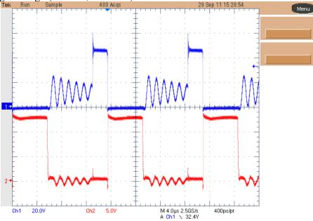
Channel 1: Vds voltage (20 V/div, **400ns/div**, no BWL). Channel 2: Vgs voltage (5 V/div, no BWL).
