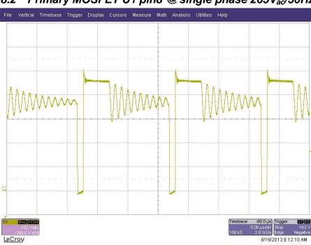
8.2 Primary MOSFET U1 pin8 @ single phase 265Vac/50Hz
