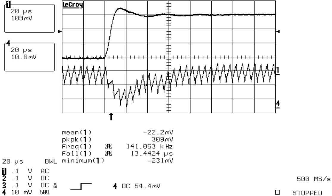
Load dump response: 48Vin and DC load of 6A off the 30Vout; additional 6A removed at about -1A per usec:
