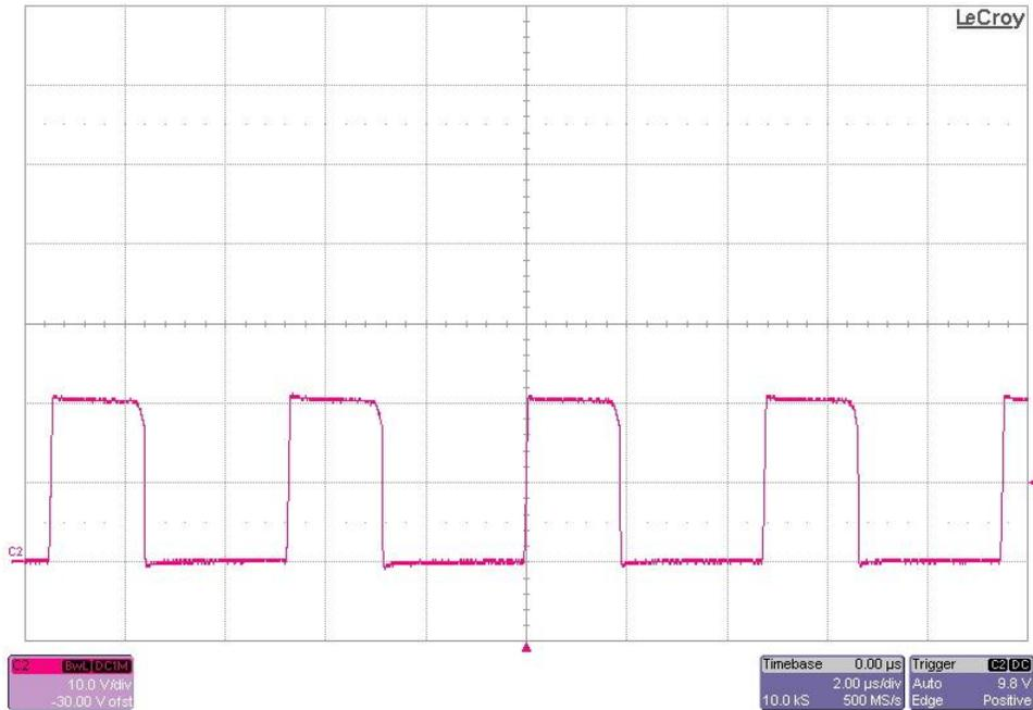
The photo below is the N-ch FET drain waveform. The input voltage is 48V and the output is loaded to 1A. (10V/DIV, 2uS/DIV)
