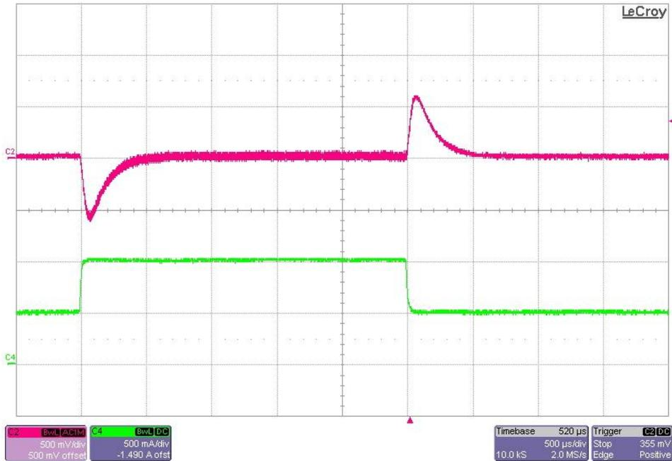
The photo below shows the 12V output voltage (top, ac coupled) when the load current is stepped between 0.5A to 1A.  $V_{in} = 48V_{dc}$  (500mV/DIV, 500mA/DIV, 500uS/DIV)
