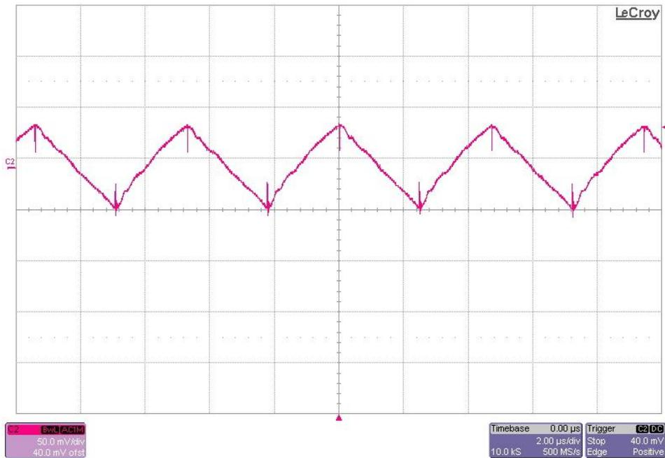
The 12V output ripple voltage is shown in the figure below. The image was taken with the output loaded to 1A and the input voltage set to 48Vdc. (50mV/DIV, 2uS/DIV)
