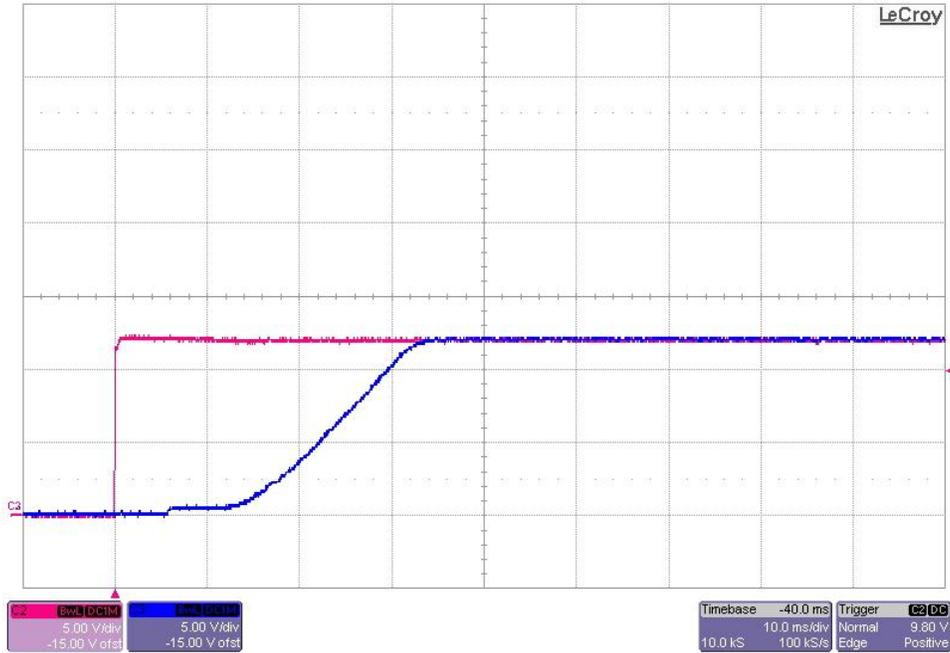
The photo below shows the 12V output voltage startup waveforms after the application of 12Vdc in. The output was loaded with a 1A resistive load. (Vin is 5V/DIV, Vout is 5V/DIV, 10mS/DIV)
