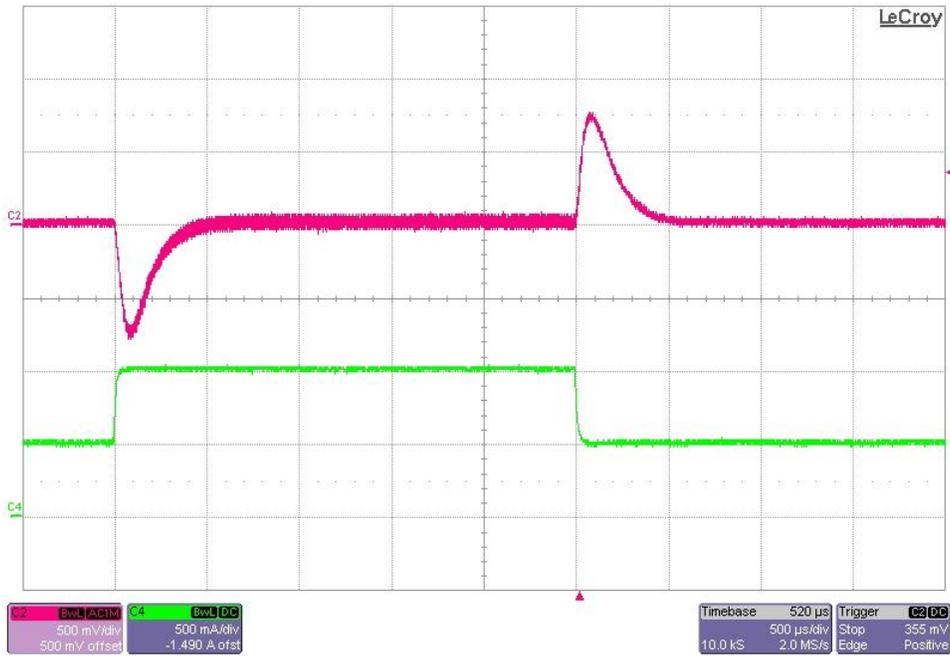
The photo below shows the 12V output voltage (top, ac coupled) when the load current is stepped between 0.5A to 1A.  $V_{in} = 12V_{dc}$  (500mV/DIV, 500mA/DIV, 500uS/DIV)
