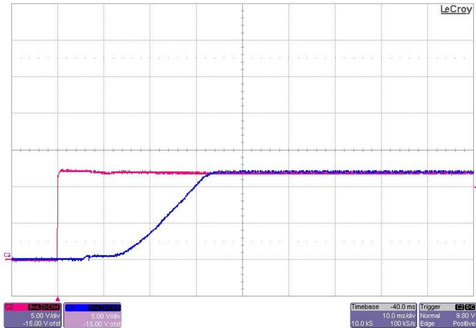
The photo below shows the 12V output voltage startup waveforms after the application of 48Vdc in. The output was loaded with a 0A resistive load. (Vin is 10V/DIV, Vout is 5V/DIV, 10mS/DIV)
