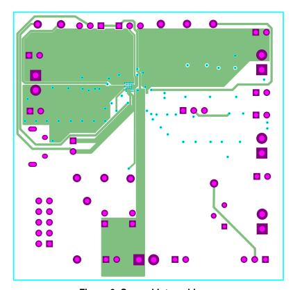
Figure 9. Second Internal Layer
