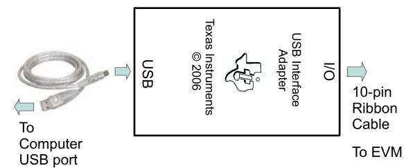
Figure 3. Connections of HPA172 Kit
