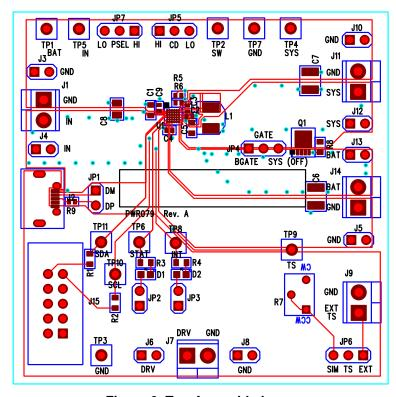
Figure 6. Top Assembly Layer
