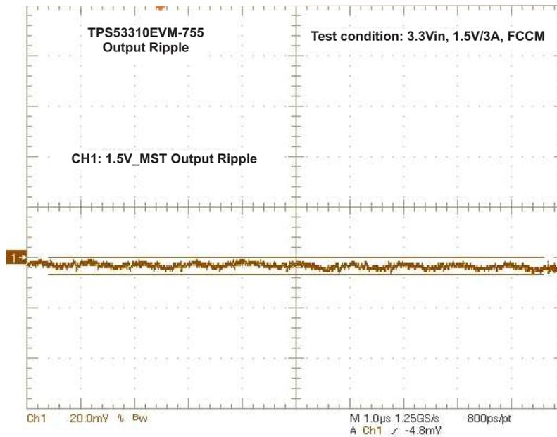
Figure 7. TPS53310EVM-755 Output Ripple (3.3 V<sub>in</sub>, 1.5 V/3 A)
