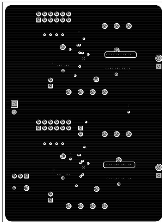
**Figure 22. TPS53310EVM-755 Internal Layer 3, Top View**
