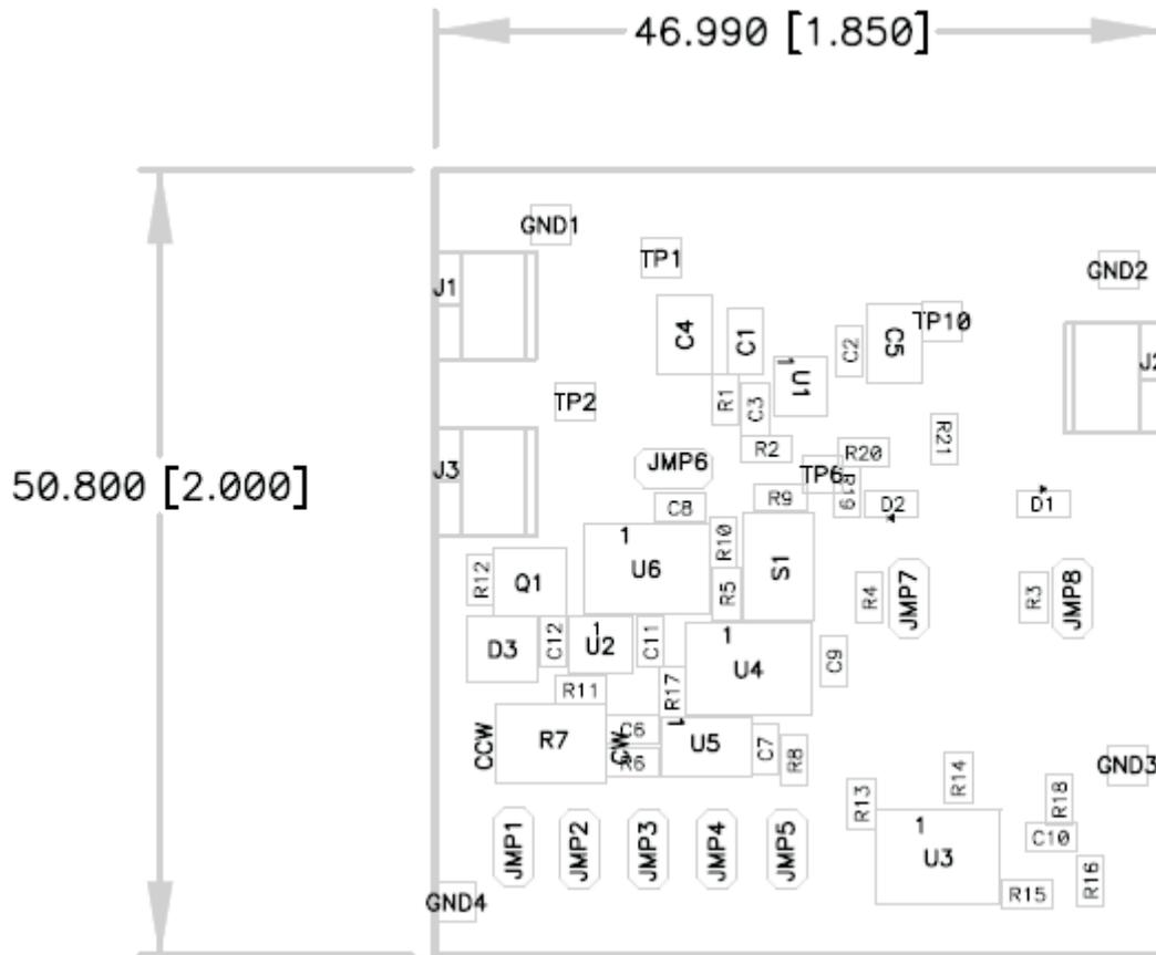
Figure 7. Assembly Layer
