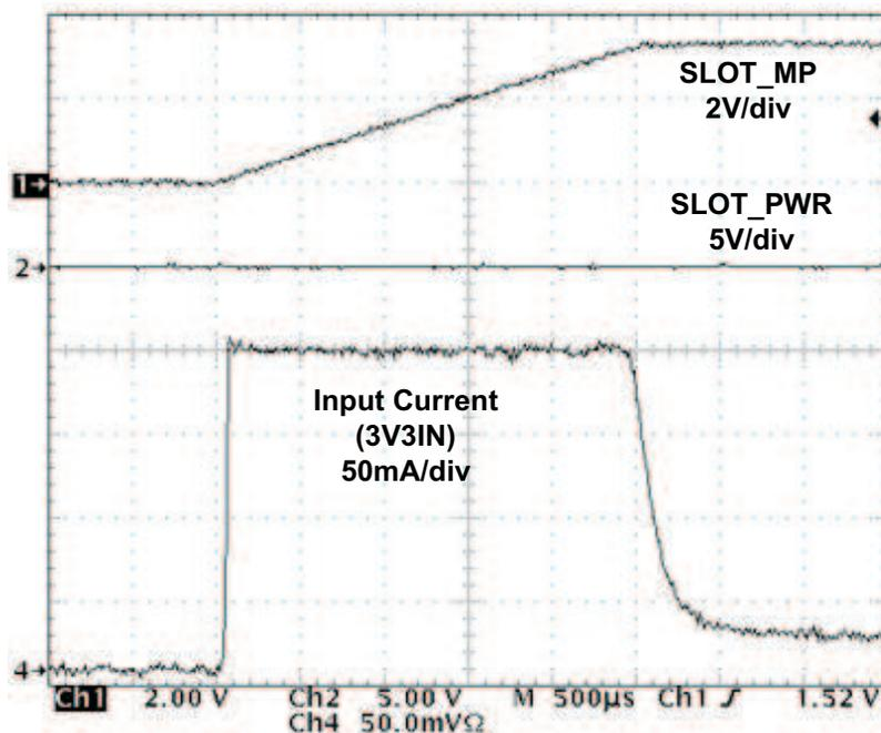
Figure 5. Output Ramp-Up waveforms - SLOT\_MP Rail.
