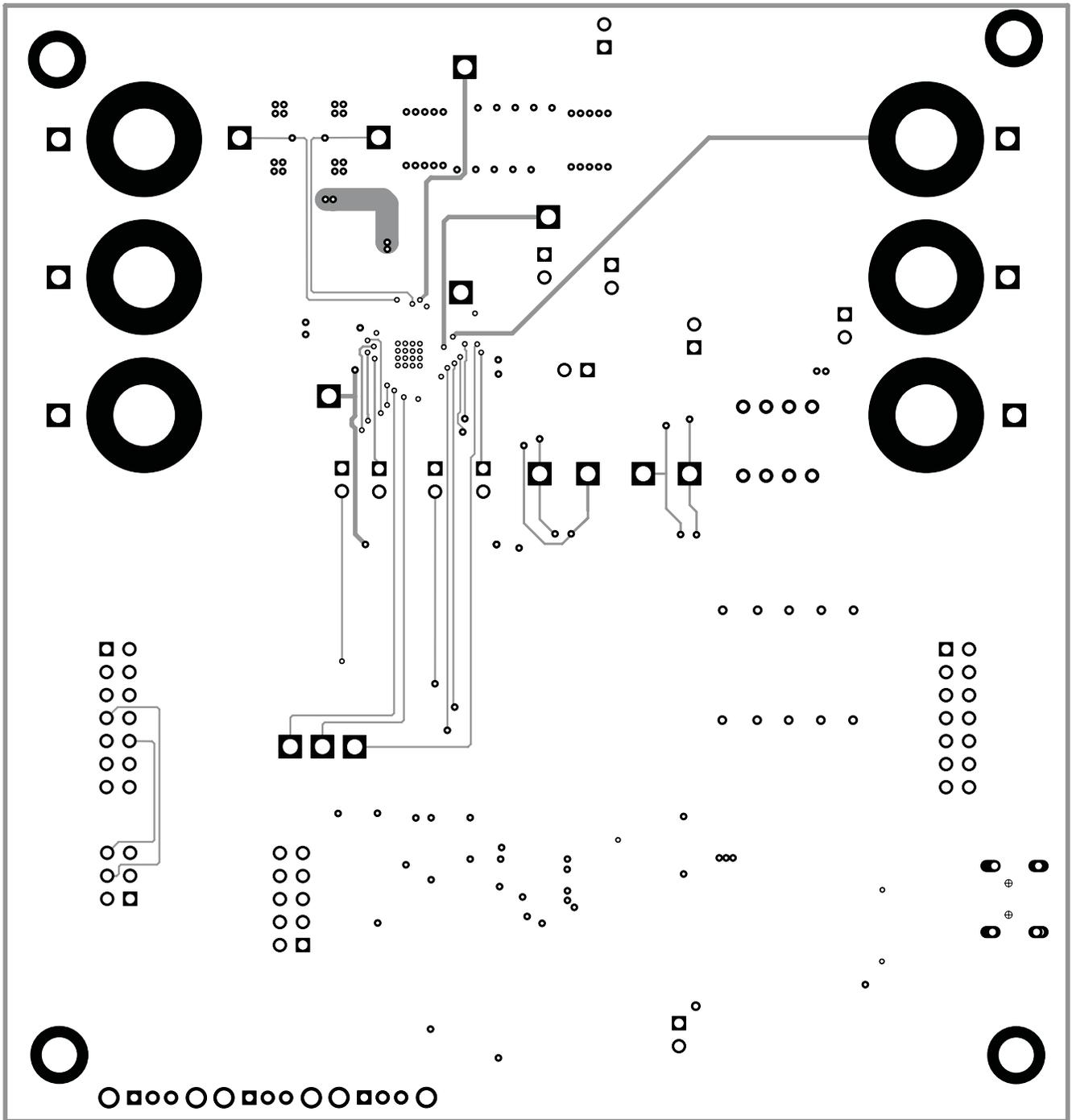
Figure 11. Layer 3 Routing
