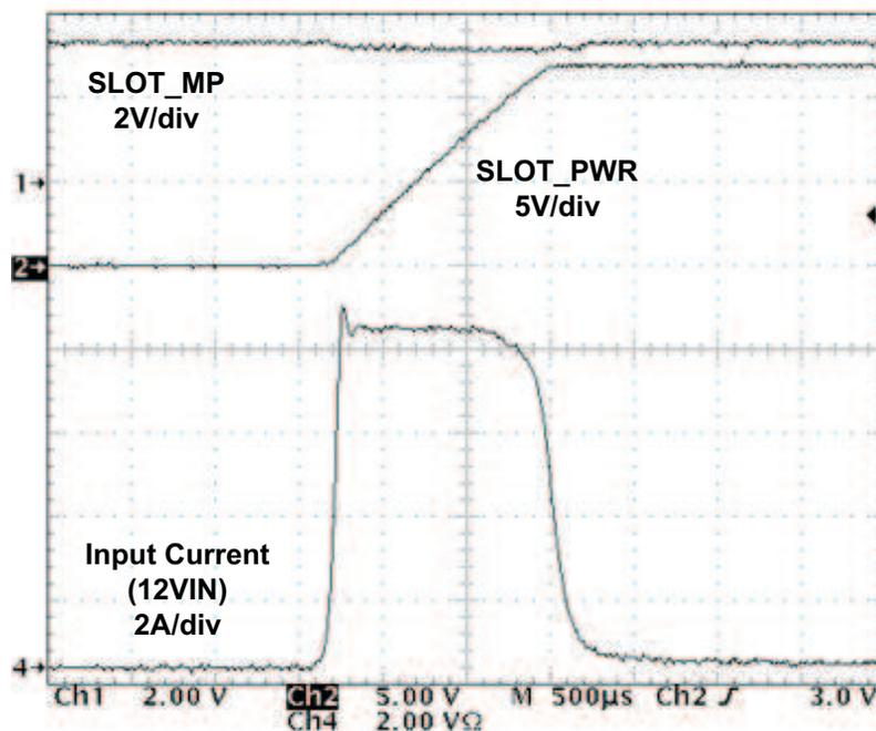
Figure 6. Output Ramp-Up Waveforms - SLOT\_PWR Rail.
