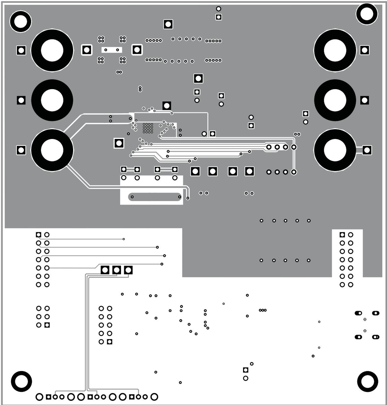
Figure 10. Layer 2 Routing
