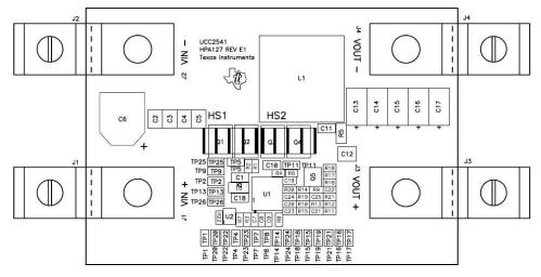
Figure 3. Test Points for HPA127 Evaluation (TOP)
