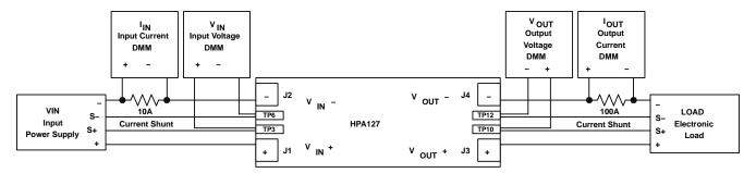
Figure 2. Recommended EVM test configuration.
