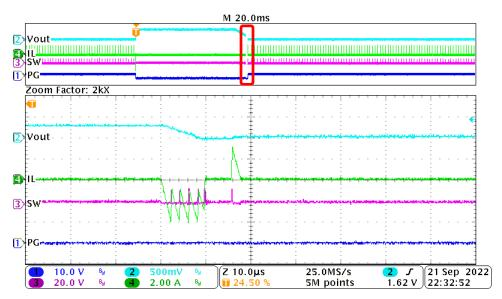
Figure 3-7. The Waveform of OOB Behavior when >OV Triggered (Zoom-in Vout Falling Waveform)
