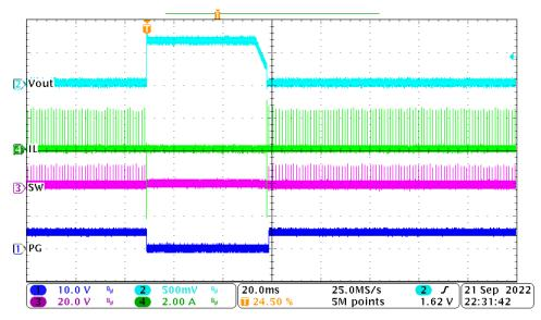
Figure 3-5. The Waveform of OOB Behavior when >OV Triggered (Full Waveform)
