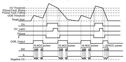
Figure 3-4. The Logic of OOB Behavior when >OV Triggered
