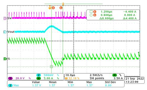
Figure 4-2. TPS56C230 Load Transient (with OOB)
