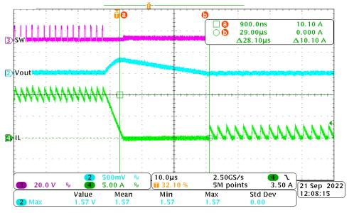
Figure 4-1. TPS51397A Load Transient (without OOB)
