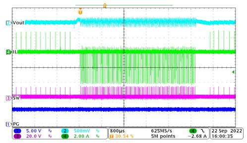
Figure 3-2. Bench Waveform of OOB Behavior when <OV Triggered (Full Waveform)
