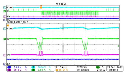
Figure 3-3. Bench Waveform of OOB Behavior when <OV Triggered (Zoom-in Waveform)
