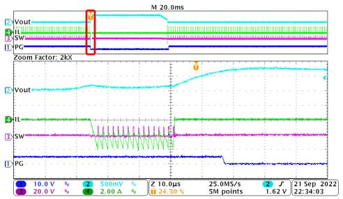
Figure 3-6. The Waveform of OOB Behavior when >OV Triggered (Zoom-in Vout Rising Waveform)
