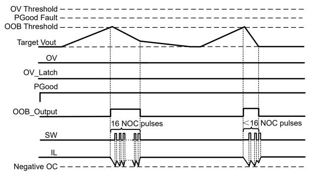
Figure 3-1. The Logic of OOB Behavior when <OV Triggered
