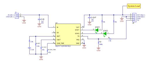
Figure 5-1. LiFePO4 45-mA Fast Charge Design
