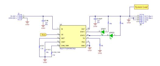
Figure 4-1. NiMH 200-mA Time Charge Design
