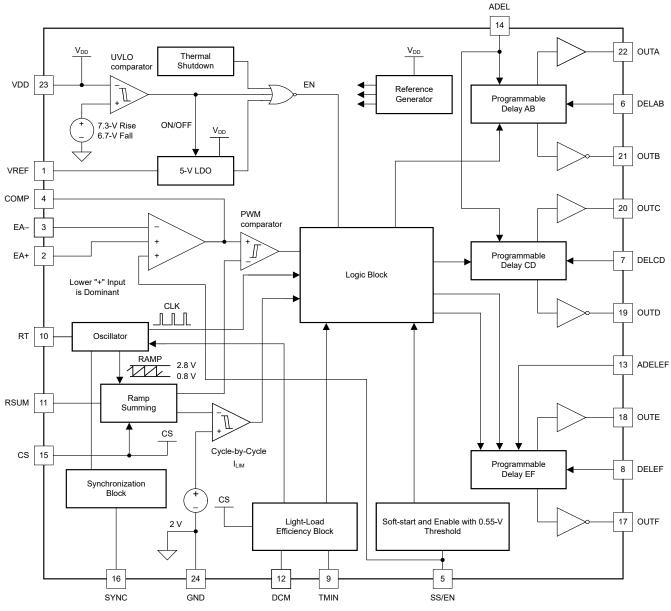
Figure 1-1. Functional Block Diagram
