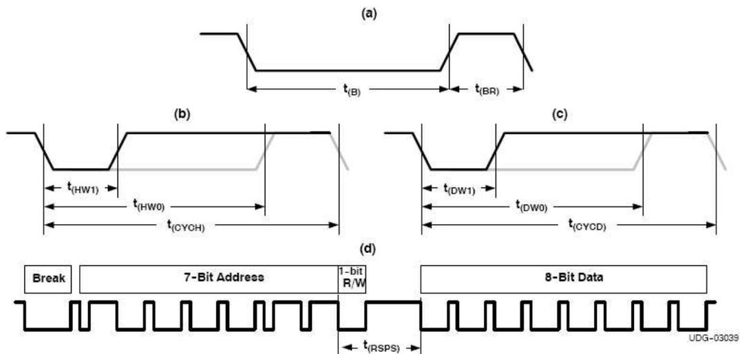
Figure 1-1. HDQ Timing Requirements
