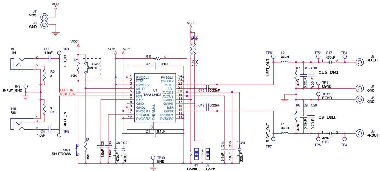
Figure 3. TPA3124D2EVM Schematic
