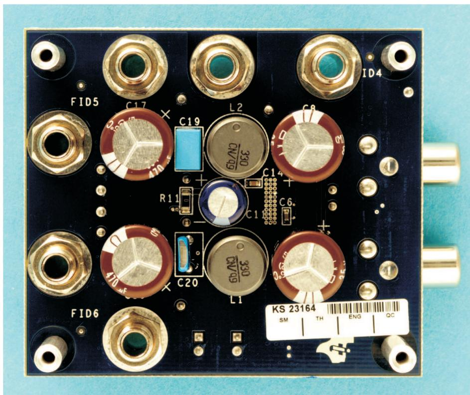
Figure 2. TPA3124D2 Audio Power Amplifier EVM – Bottom View
