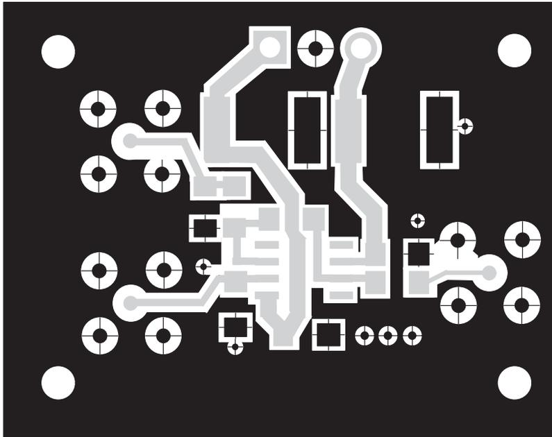
Figure 2–3. THS4081 EVM PC Board Layout: Back Side
