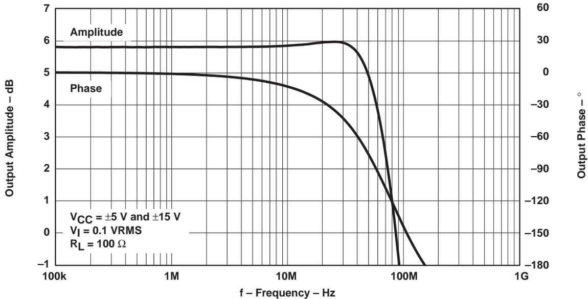
Figure 1–4 shows the typical frequency response of the THS4081 EVM using the inverting input ( $G = -1$ ). Typical  $-0.1$  dB bandwidths are 25 MHz and a  $-3$ -dB bandwidth of 65 MHz with a  $\pm 15$  V power supply. These bandwidths remain consistent when the power supply drops to  $\pm 5$  V.
