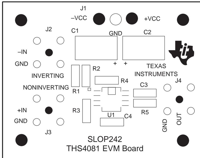
Figure 2–2. THS4081 EVM PC Board Layout: Component Side
