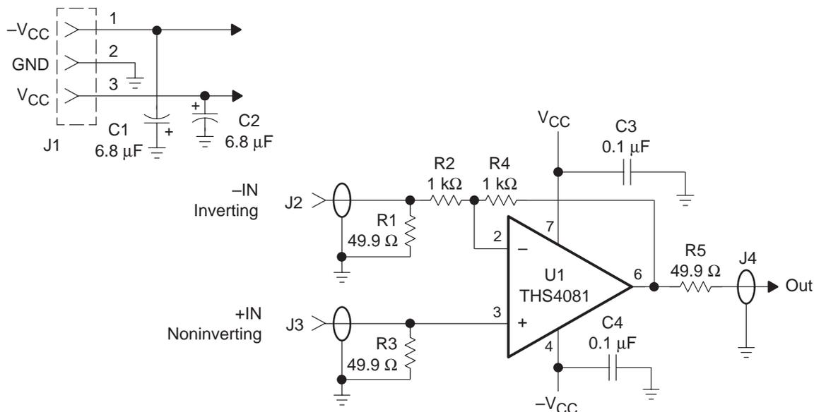
The gain of the EVM inputs can easily be changed to support a particular application by simply changing the ratio of resistors R1, R4, and R5 as described in the following equations:
