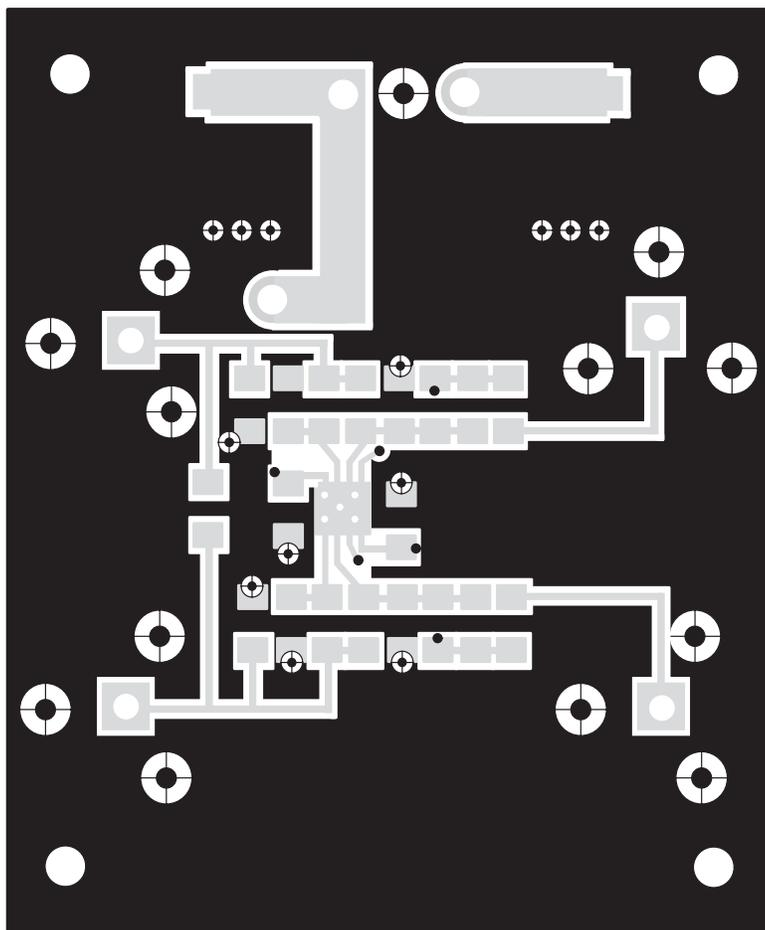
Figure 2–4. THS6062 EVM PC Board Layout – Back Side
