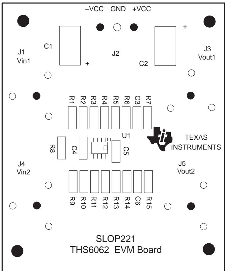
Figure 2–3. THS6062 EVM PC Board Layout – Component Side
