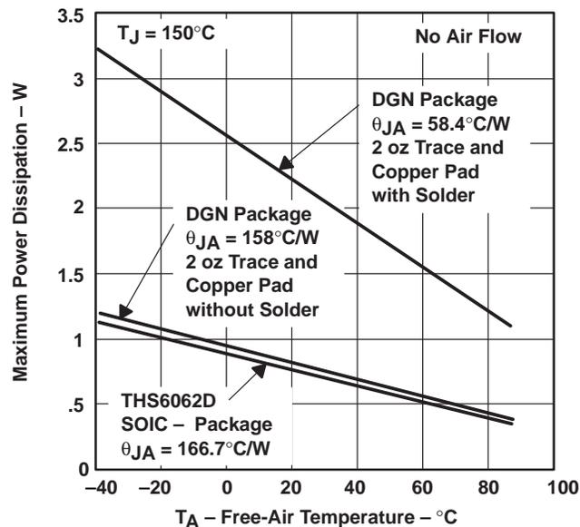
Even though the THS6062 EVM PCB is smaller than the one in the example above, the results should give an idea of how much power can be dissipated by the PowerPAD IC package. The THS6062 EVM is a good example of proper thermal management when using PowerPAD-mounted devices.
