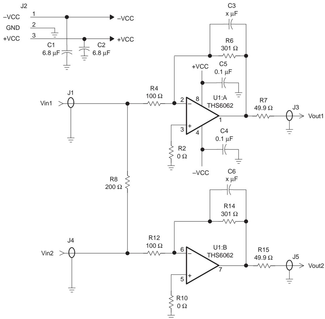
The gain of the EVM inputs can easily be changed to support a particular application by simply changing the ratio of resistors R6 and R4 (channel 1) and R14 and R12 (channel 2) as described in the following equation:
