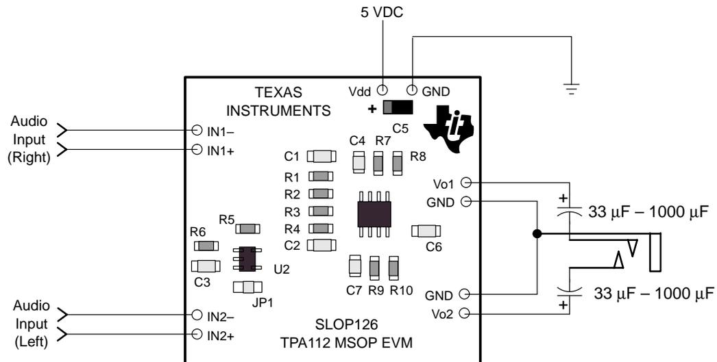
† Due to the very small size of the MSOP IC package, the standard part number TPA112 is replaced with the code TIAAD
