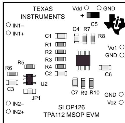
† Due to the very small size of the MSOP IC package, the standard part number TPA112 is replaced with the code TIAAD
