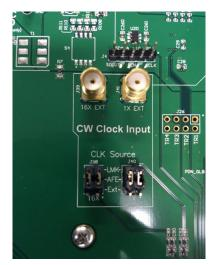
Figure 8. AFE58xxx8 Default CW Jumper Configuration
