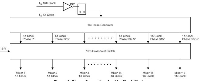
Figure 2. Phase Generation for 16× Clock Mode
