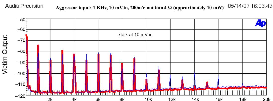
**Figure 8. Channel 1 → Channel 3 Harmonic Crosstalk With Default Switching Phase Settings**
