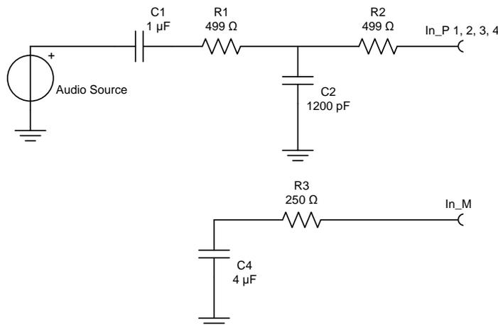
Figure 1. TAS5414C Input Circuit
