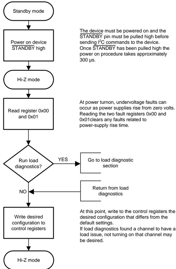
**Figure 10. Power Up and Initialization**
