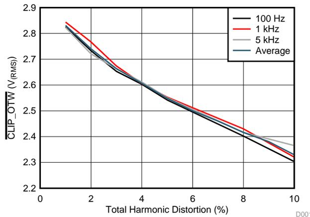
Figure 6. CLIP\_OTW Pin Voltage Versus % of THD
