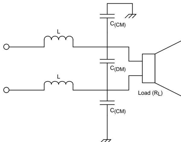
Figure 4. Typical Output Demodulation Filter
