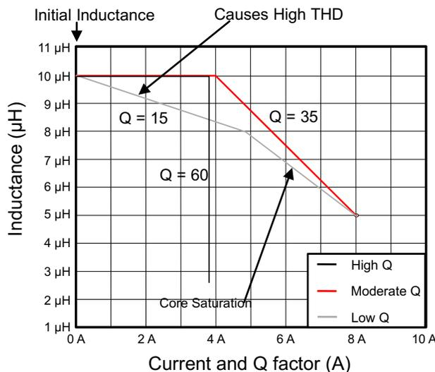
**Figure 5. Inductance Versus Current and Q Factor**
