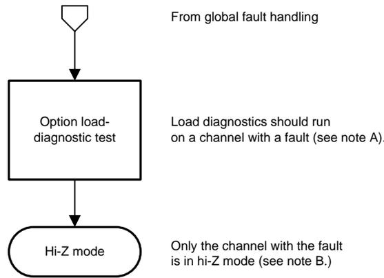
Figure 15. Channel Fault Handling
