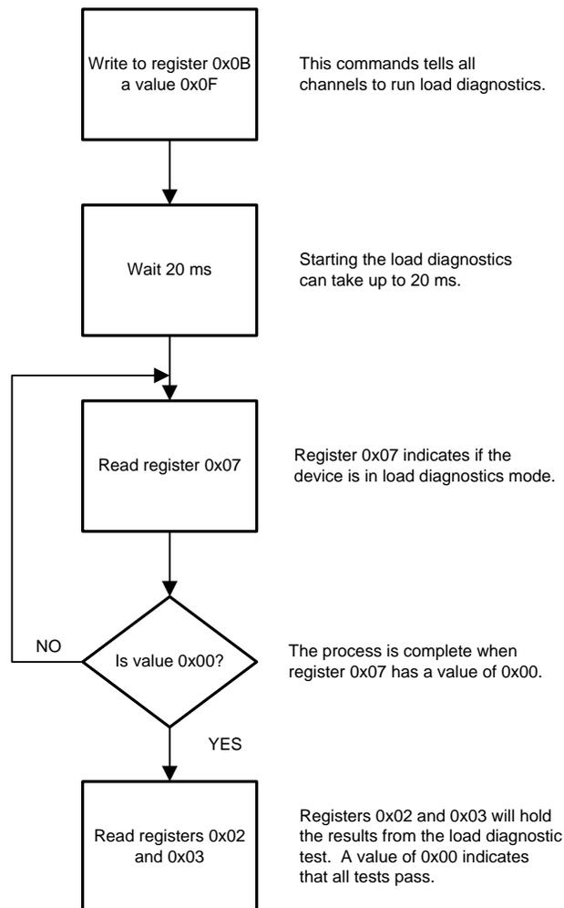
**Figure 13. Load Diagnostics, Four Channels**
