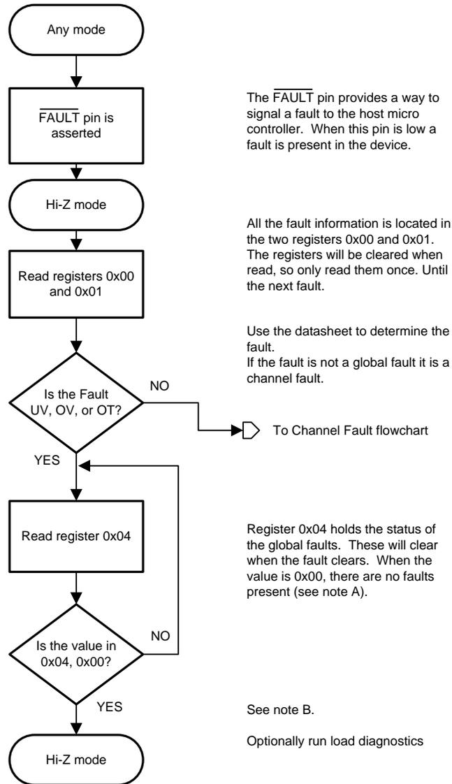
Figure 14. Global Fault Handling
