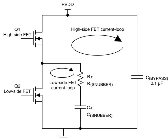
**Figure 3. One-Half of the Typical Output Stage With Snubbers**
