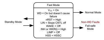
Figure 2-6. Fast Mode in Pin Control
