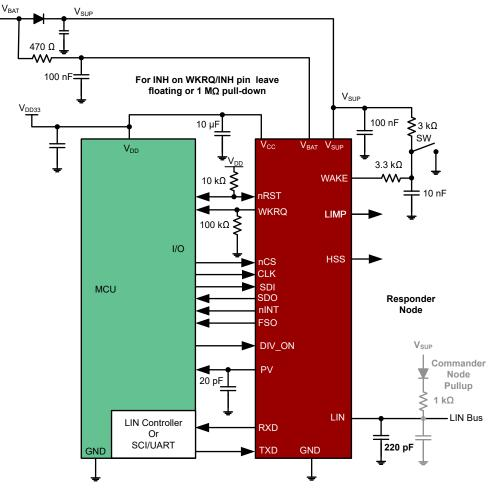
Figure 3-1. Typical Application of TLIN1431-Q1 in SPI Control
