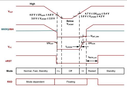
Figure 1-5. Brownout below V<sub>nPORF</sub>
