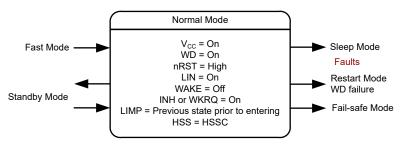
Figure 2-5. Normal Mode in Pin Control
