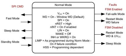
Figure 3-5. Normal Mode in SPI Control
