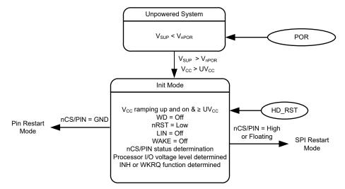
Figure 1-4. INIT Mode State Diagram
