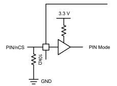
Figure 1-1. PIN/nCS Configuration for Pin Control
