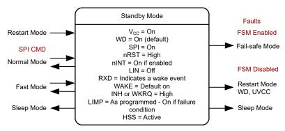
Figure 3-4. Standby Mode in SPI Control
