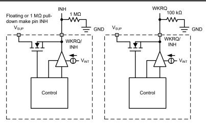
Figure 1-3. WKRQ/INH Pin Configurations
