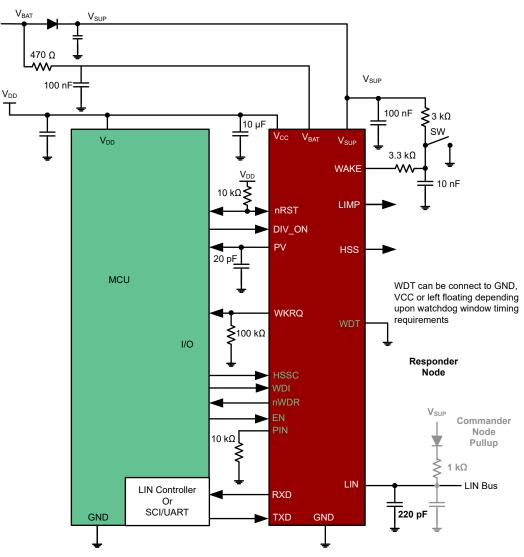
Figure 2-1. Typical Application of TLIN1431-Q1 in Pin Control
