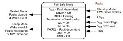
Figure 2-9. Fail-Safe Mode in Pin Control
