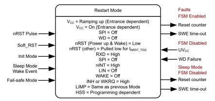
Figure 3-3. Restart Mode in SPI Control
