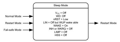
Figure 2-8. Sleep Mode in Pin Control
