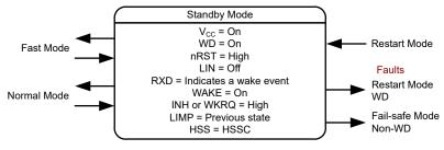
Figure 2-4. Standby Mode in Pin Control
