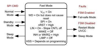
Figure 3-6. Fast Mode in SPI Control
