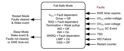
Figure 3-8. Fail-Safe Mode in SPI Control
