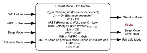
Figure 2-3. Restart Mode in Pin Control
