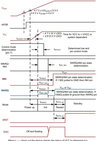
When  $t_{\text{LDOON}}$  times out the device checks the status of VCC to determine if a short or over-voltage is present. VCC may or may not have reach regulation
