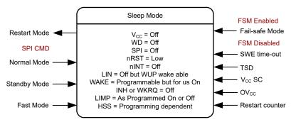
Figure 3-7. Sleep Mode in SPI Control
