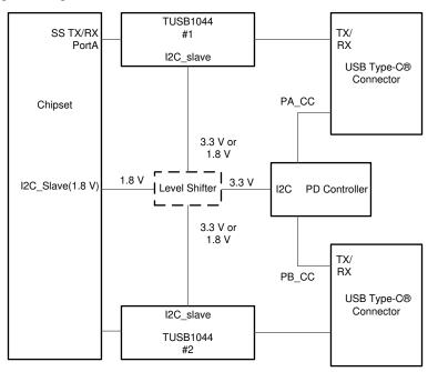
Figure 5-1. TUSB1044 Block Diagram in a DFP System
