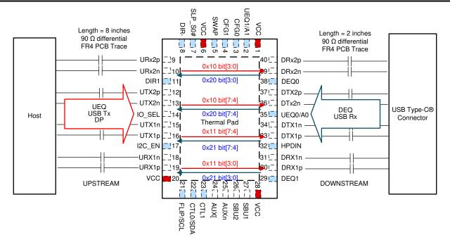
Figure 2-2. Reference Block Diagram for TUSB1044 Equalization Control
