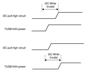
Figure 6-5. Example of Invalid I<sup>2</sup>C Write Region
