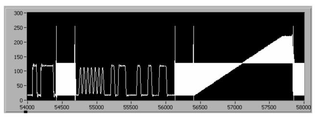
Figure 2. TVP5150A Line 21 Closed Caption ITU-R BT.656 Digital Output Capture in Raw Data Mode. UV (chroma) data are replaced with Y (luma) data.
