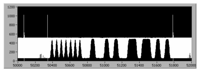
Figure 3. TVP5146 Line 21 Closed Caption ITU-R BT.656 Digital Output Capture With YUV Samples Present. Raw Data Mode is disabled.
