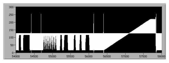
Figure 1. TVP5150A Line 21 Closed Caption ITU-R BT.656 Digital Output Capture With YUV Samples Present. Raw Data Mode disabled.
