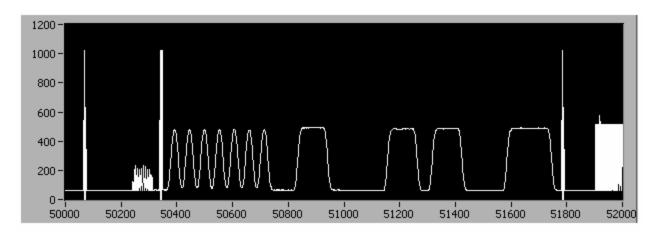
Figure 4. TVP5146 Line 21 Closed Caption ITU-R BT.656 Digital Output Capture in Raw Data Mode. UV (chroma) data are replaced with Y (luma) data.
