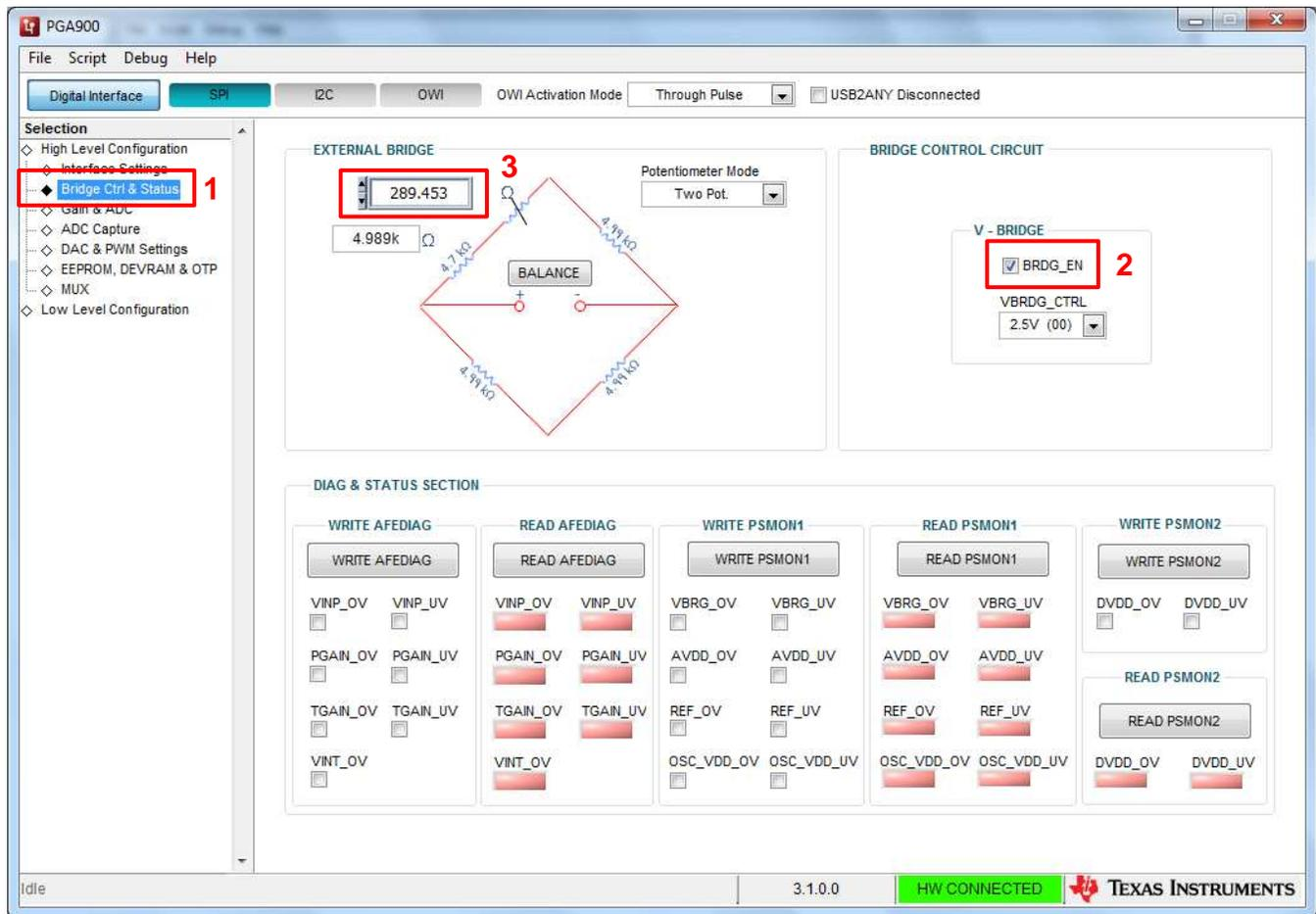
Figure 5. Enabling Bridge Voltage in PGA900 and Configuring Resistive Bridge in PGA900EVM
