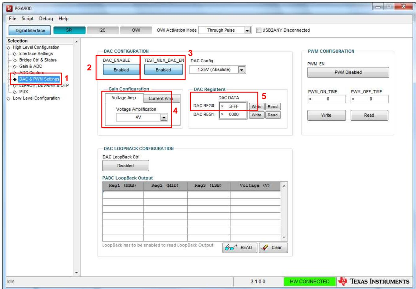
Figure 7. Writing Directly to the DAC in the PGA900
