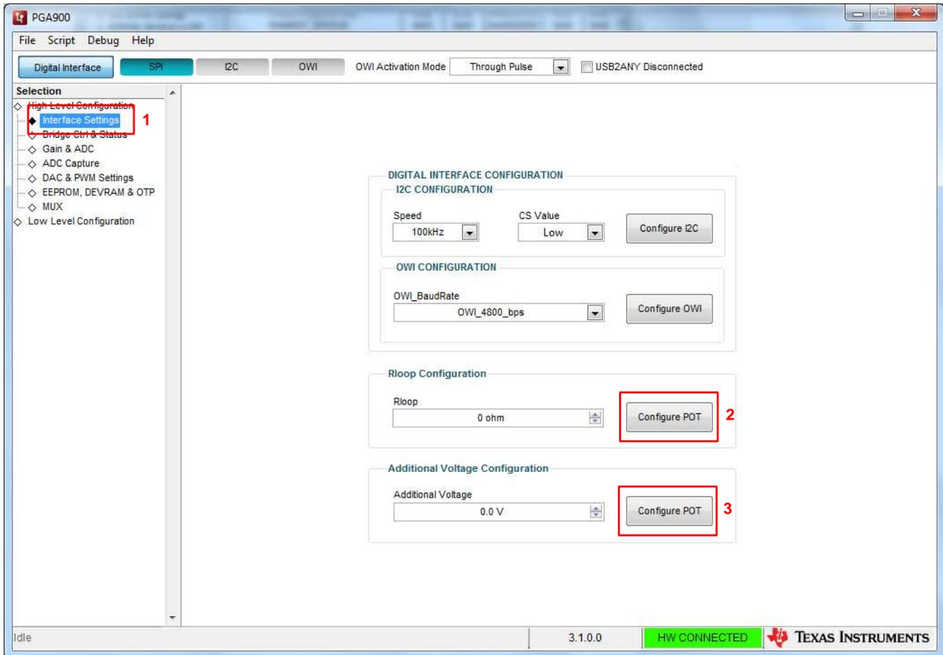
Figure 2. Configuring the Hardware for Voltage Mode
