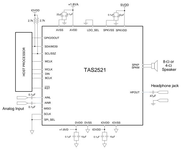
Figure 1-2. Typical Circuit Configuration
