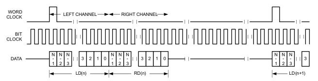
Figure 2-20. Timing Diagram for DSP Mode With Offset = 0 and Bit Clock Inverted
