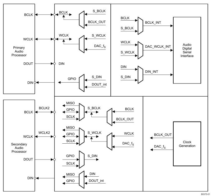
Figure 2-21. Audio Serial Interface Multiplexing
