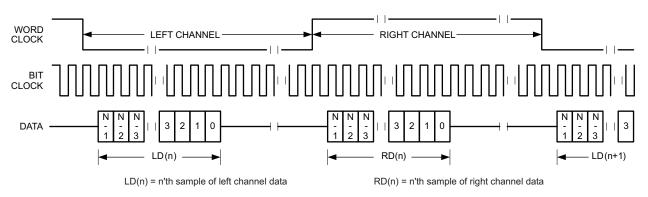
Figure 2-17. Timing Diagram for I<sup>2</sup>S Mode With Offset = 0 and Bit Clock Inverted
