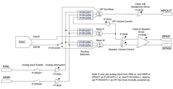
Figure 2-6. Analog Block Diagram
