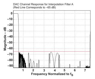
Figure 2-3. Frequency Response of DAC Interpolation Filter A
