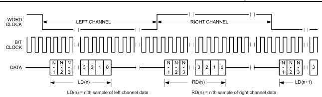
Figure 2-15. Timing Diagram for I<sup>2</sup>S Mode
