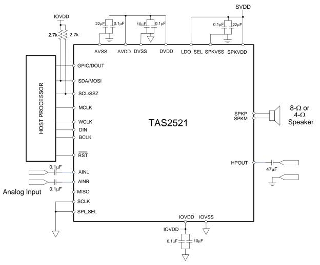
Figure 1-3. Application Schematics for LDO
