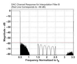
Figure 2-4. Frequency Response of Channel Interpolation Filter B
