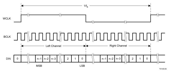
Figure 2-11. Timing Diagram for Right-Justified Mode
