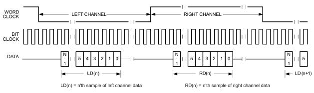
Figure 2-16. Timing Diagram for I<sup>2</sup>S Mode With Offset = 2
