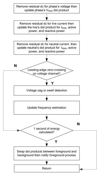
Figure 10. per\_sample\_dsp() for Neutral-Monitoring Configuration
