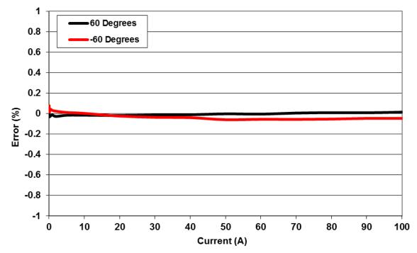
Figure 37. Channel B Reactive Energy Measurement Error, Common-Voltage
