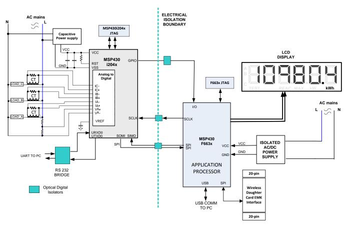
Figure 1. EVM430-i2040 System Block Diagram for Common-Voltage Configuration
