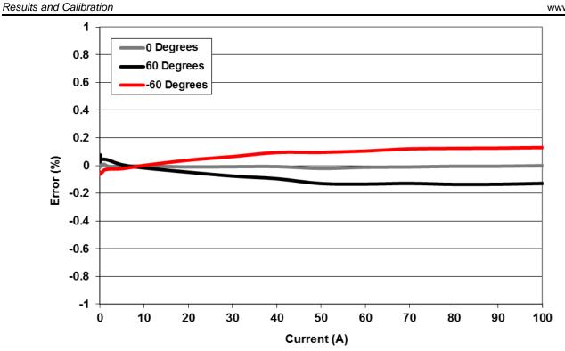
Figure 38. Channel C Active Energy Measurement Error, Common-Voltage
