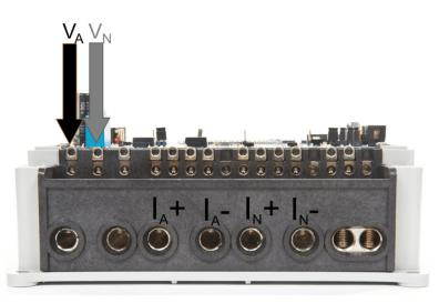
Figure 20. Front View of the EVM With Test Setup Connections, Neutral-Monitoring
