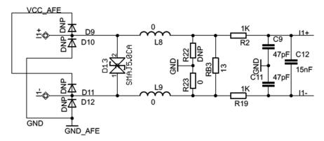
Figure 7. Analog Front End for Current Inputs
