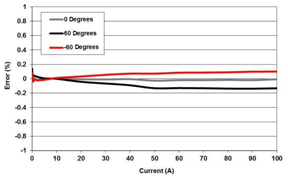
Figure 34. Channel A Active Energy Measurement Error, Common-Voltage
