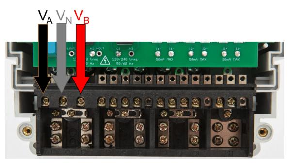
Figure 18. Top View of EVM with Test Setup Connections, Two-Phase
