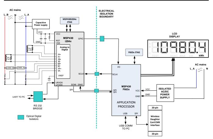
Figure 3. EVM430-i2040 System Block Diagram for Two-Phase Configuration
