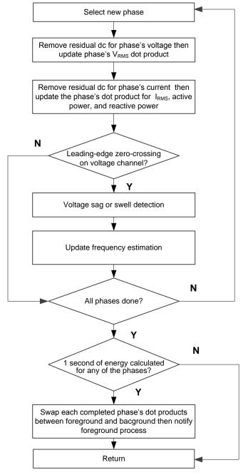
Figure 12. per\_sample\_dsp() for Two-Phase Configuration
