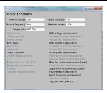
Figure 33. Meter Features Window
