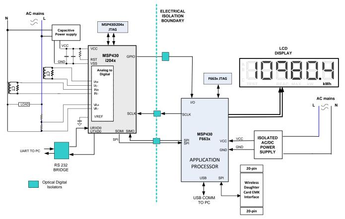
Figure 2. EVM430-i2040 System Block Diagram for Neutral-Monitoring Configuration
