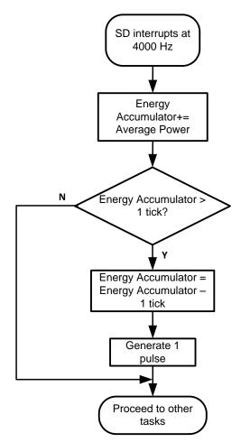
Figure 14. Pulse Generation for Energy Indication
