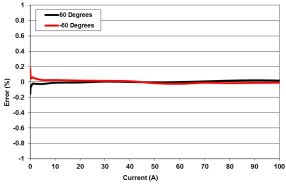
Figure 35. Channel A Reactive Energy Measurement Error, Common-Voltage
