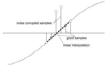
Figure 13. Frequency Measurement
