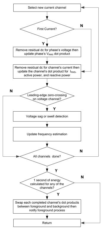
Figure 11. per\_sample\_dsp() for Common-Voltage Configuration
