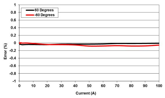
Figure 41. Cumulative Phase Reactive Energy Measurement Error, Two-Phase
