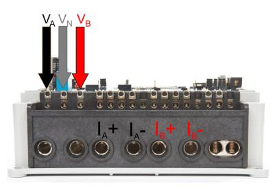
Figure 21. Front View of the EVM With Test Setup Connections, Two-Phase
