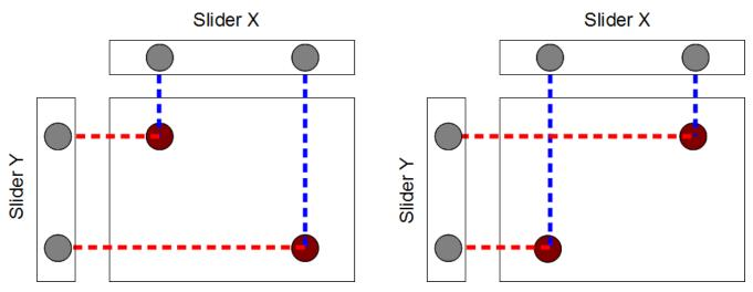
Figure 12. Example of Same Measuring Result of Different Finger Positions
