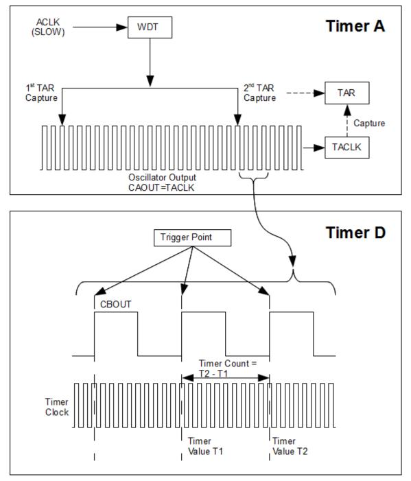
Figure 4. Measurement of Waveform Using Timer\_A vs Timer\_D
