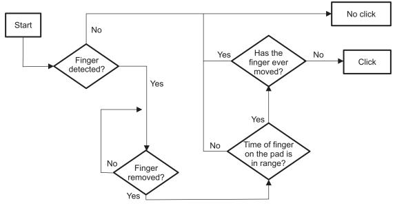
Figure 13. Flowchart of Determination of a Mouse Click
