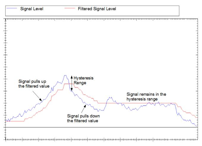
Figure 9. Filtering Signal Level Using Hysteresis
