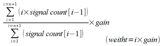
Figure 10. Weighted averaging for calculating position.
