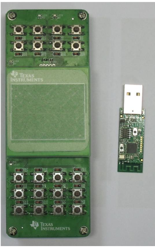
Figure 20. The Remote Control and the USB Receiver
