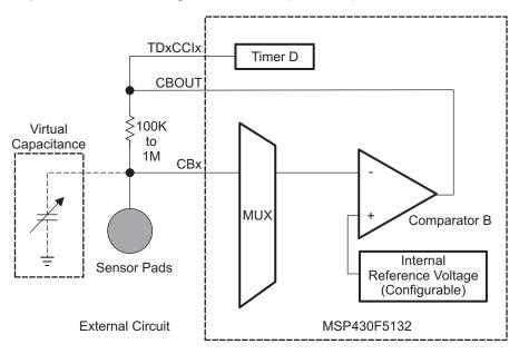
Figure 2. Single Sensor Block Diagram
