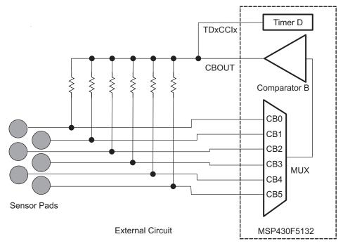
Figure 5. Multiple Sensor Block Diagram
