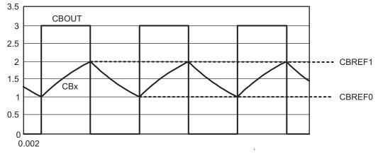
Figure 3. Waveform of CBOUT and the Sensor
