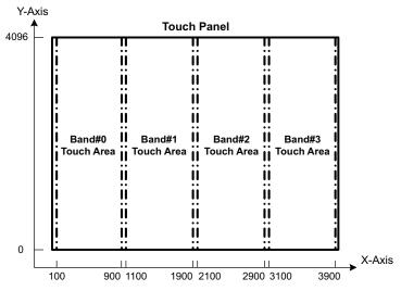
Figure 3. Divide TS or Touch Panel for Scroll Bars
