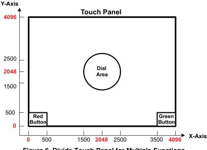
Figure 6. Divide Touch Panel for Multiple Functions
