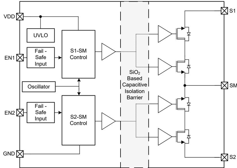
**Figure 1-1. TPSI2072-Q1 Functional Block Diagram**
