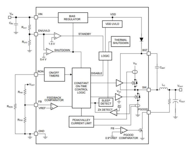
Figure 1-1. Functional Block Diagram
