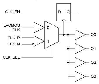
Figure 1-1. Functional Block Diagram
