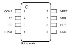
Figure 4-1. Pin Diagram SOIC (8) Package
