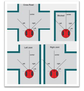
Figure 1. As the robot is exploring the maze, it encounters these eight possible scenarios. When the robot approaches an intersection, it first determines what alternative paths exist, and then it chooses which way to go
