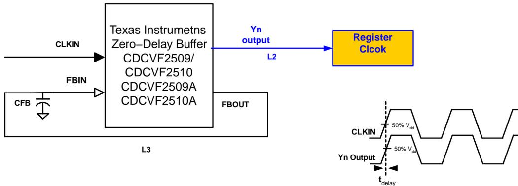
Figure 1. L2=L3, Zero Phase Delay Between CLKIN and Yn
