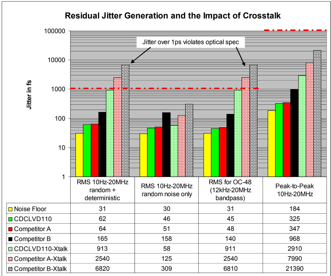
**Figure 5. PN9000 Phase Jitter Measurements**
