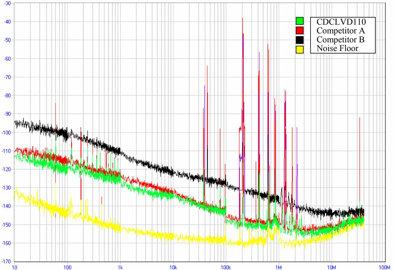
**Figure 7. Crosstalk Phase Noise Comparison at 622.08 MHz**
