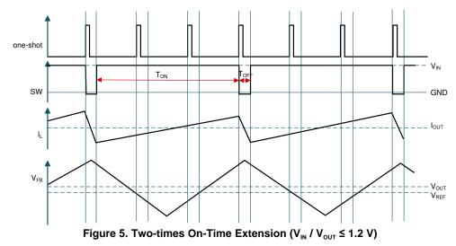
Table 1 shows the detailed summary. For the TPS568230 device, when the  $V_{IN} / V_{OUT} \le 1.2$ , the switching frequency is designed to drop to about 500 kHz.
