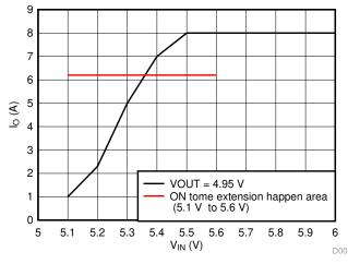
Figure 12. TPS568230 V<sub>IN</sub> vs I<sub>o</sub> Curve
