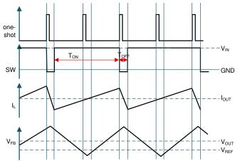
Figure 4. One-time On-Time Extension (1.2 V < V<sub>IN</sub> / V<sub>OUT</sub>  $\leq$  1.6 V)
