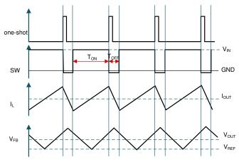
Figure 3. Normal Operation Without On-Time Extension
