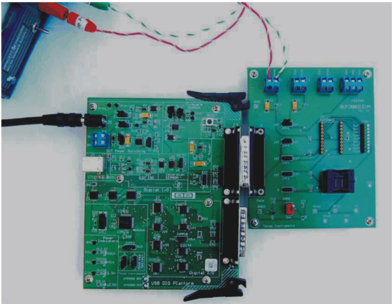
Figure 5. Connecting External Power to the EVM
