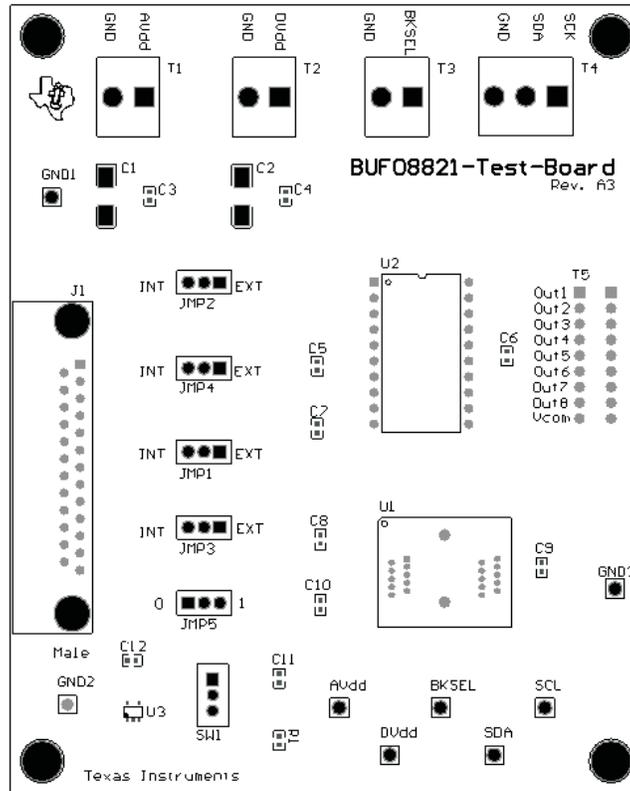
**Figure 23. BUF08821EVM-USB PCB Top Layer (Component Side)**
