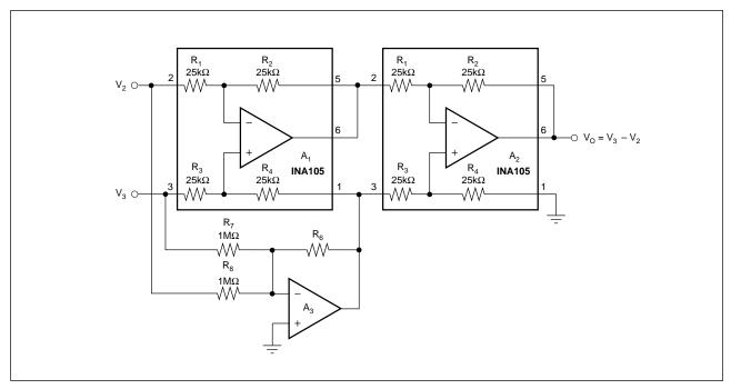
FIGURE 6. Boosting the INA105 Common-Mode Input Range Dynamically.
