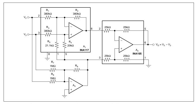
FIGURE 5. Boosting the INA117 Common-Mode Input Range Dynamically.
