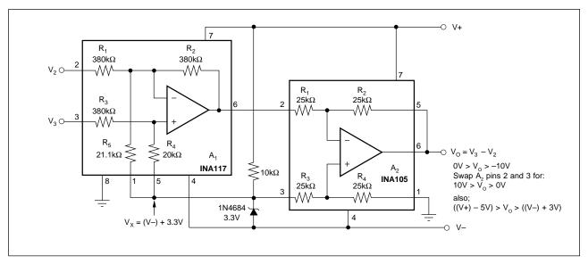
FIGURE 2. Offsetting the INA117 Common-Mode Input Range with a Zener Reference.
