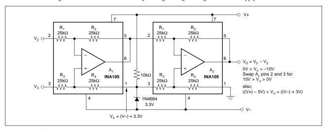
FIGURE 4. Offsetting the INA105 Common-Mode Input Range with a Zener Reference.
