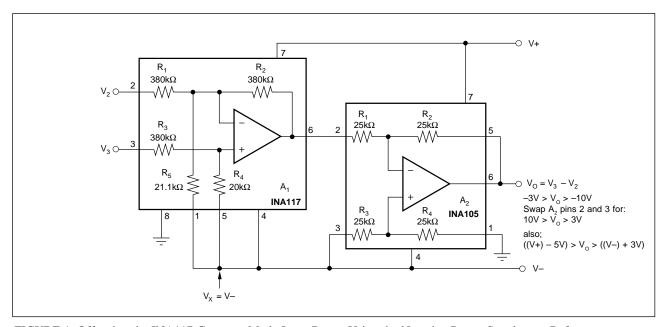
FIGURE 1. Offsetting the INA117 Common-Mode Input Range Using the Negative Power Supply as a Reference.
