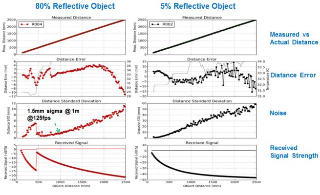
Figure 2. OPT3101 EVM Based Measurements
