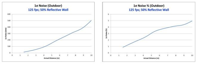
Figure 12. 1<sup>st</sup> Noise vs Distance (Outdoor)
