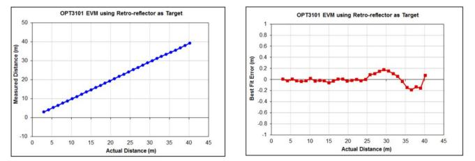
Figure 14. Measurement Distance vs Actual Distance
