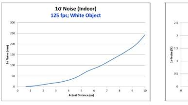
Figure 8. 1<sub>o</sub> Noise vs Distance (Indoor)
